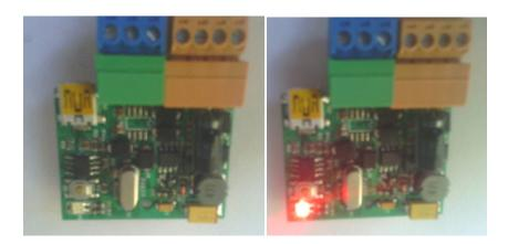
Long press Broadcast button until red light on, then click detect address from C-touch Sw. If you can find Subnet ID and Device ID then can start to configure it. (same way of programming like other smarthome items) .
